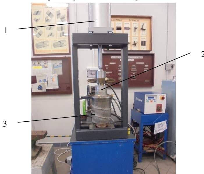
Fig. 3. Modified SPS device used in experimental research: 1 – pneumatic press; 2 – mould; 3 – vacuum chamber
